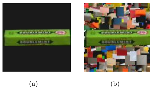
Figure 4.2: Input Images of a Single Object — The figure shows an object from the COIL-100 database (NENE et al., 1996) as (a) segmented and (b) unsegmented image. Since the images of that database are perfectly segmented, unsegmented test images were manually created before presentation by pasting the object in the segmented image into a cluttered background consisting of arbitrarily chosen image patches of random size derived from the images of the current testing set.
