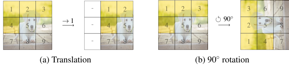
Figure 2.6: The translation group T(2) and the group of 90^\circ rotations SO(2,4) acting on two-dimensional inputs can be expressed as a permutation p of the pixels.
