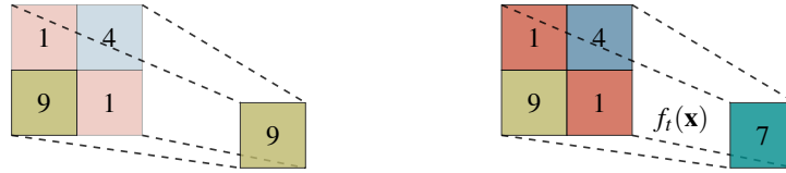
Figure 1.4: Max pooling (left) guarantees invariance, but only preserves a single value of the input space, effectively destroying the other available information. In contrast, adding targeted model capacity via an invariant extraction function f_i(\mathbf{x}) (right) is able to consider and weight all available information while still guaranteeing invariance.
