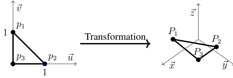
Figure 4.6: Representation of the transformation from a flat triangle in the general coordinate system to the unit triangle.
