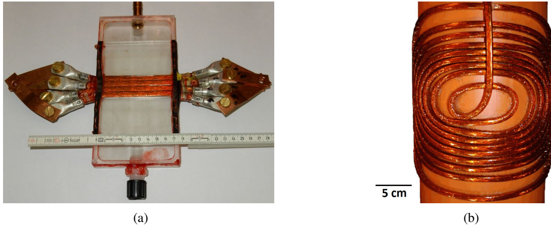
Figure 6.3: (a) Cooling model used to estimate the cooling efficiency.(b) Coil prototype used to validate the wire stiffness and the coil design.
