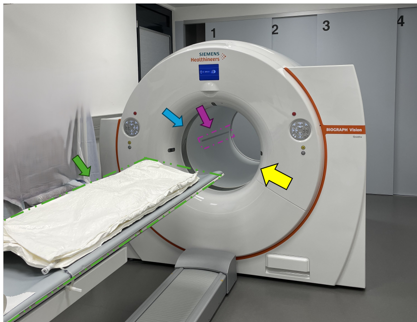
Fig. 2.5: A commercial PET/CT system showing the system's bore (yellow), patient bed (green), CT component (blue), and PET component (pink).
