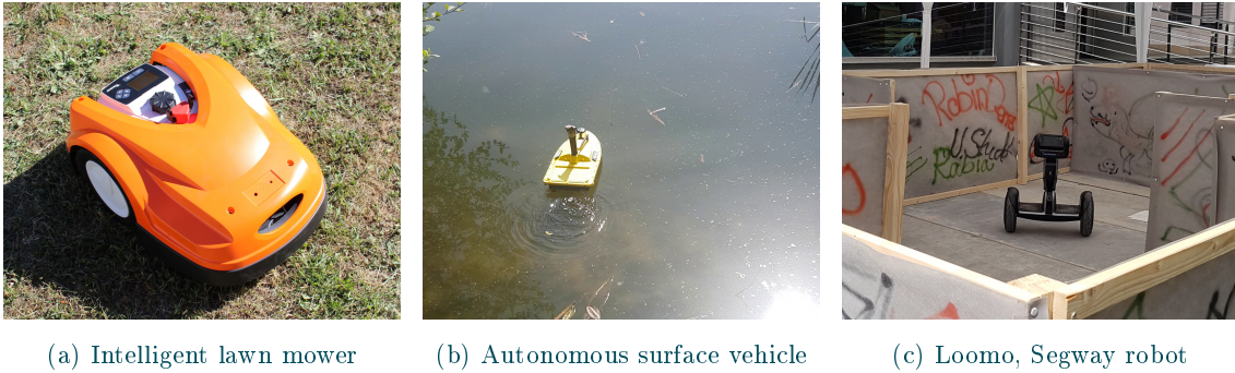
Figure 4.5: Mobile robotic platforms for which ROS-Mobile is currently used within the author’s institute. From left to right: (a) intelligent lawn mower with low-cost sensors for domestic purpose, (b) autonomous surface vehicle (ASV) for swarm approaches to monitor water contamination, (c) Loomo from Segway-Ninebot for person guidance in hospitals.
