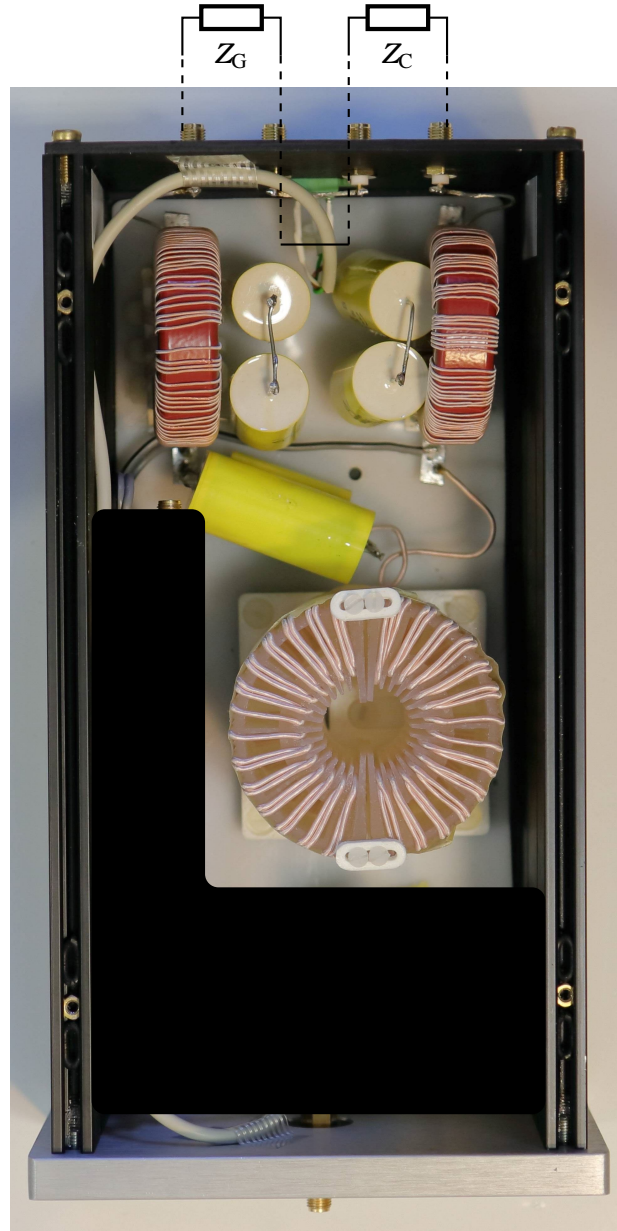
Figure 4.4: Installed BSF in the chassis. The receive coils in the generation and cancellation units are illustrated by Z_G and Z_C , respectively. Note that the BSF in each receive channel is installed in a separate chassis.
