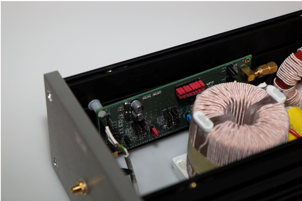
Figure 4.5: Installed LNA in the chassis. The printed circuit board (PCB) board is the self-developed LNA. It is installed together with the BSF in the same chassis. Note that the LNA in only one channel is shown.
