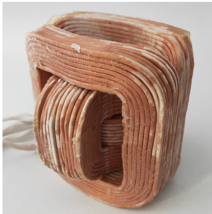
Figure 3.16: Assembly of the fabricated transmit coils. A dual-component epoxy adhesive is used to bond the wires during the winding of the coils.
