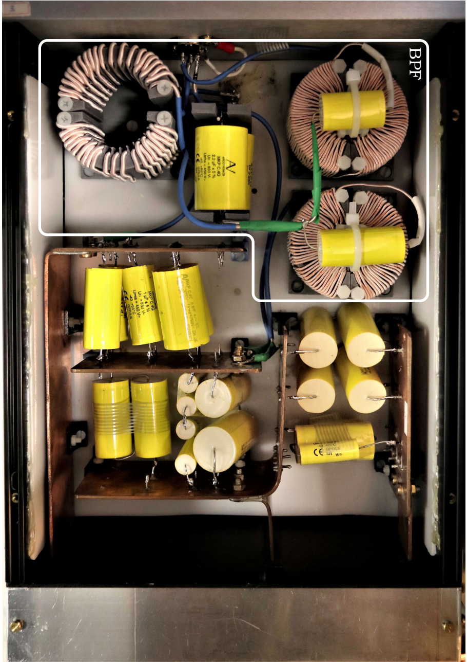
Figure 3.26: Installed BPF in the chassis. The solid frame indicates the three-order LC BPF. Note that the installed BPF in only one transmit channel is shown.
