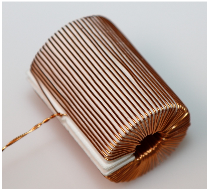
Figure 5.4: Self-built Rogowski coil. The copper wire is wound on a 3D printed coil former with a rectangular cross-section. The former has 12 mm inner radius, 15 mm outer radius, and 40 mm height.
