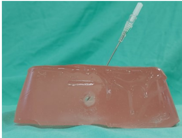
Figure 4.6: Photograph of the phantom with a placed needle to illustrate the easily identifiable successful puncture.
