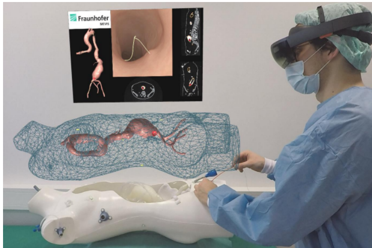
Figure 4.17: The virtual body surface (turquoise wireframe), aorta (red), catheter tip (blue sphere) and 2D panel above the torso model (white phantom without its top cover). This 2D panel displayed the aortic model, the VA image with its centerline (yellow) and the orthogonal views of the preoperative CT scan corresponding to the current position of the catheter tip (red sphere).
