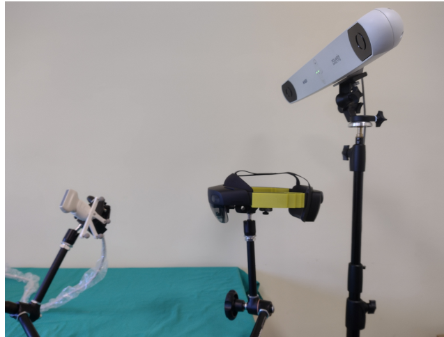
Figure 3.5: Setup for the static tracking accuracy evaluation. HoloLens 2 and the OTS are fixed, while the US probe with its marker is moved to 20 different poses for measurement acquisition.
