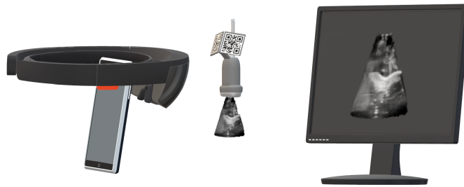
Figure 4.7: The schematic setup for measuring the latency of displayed US volumes. A slow-motion video captures the US station screen and the rendered US volume.
