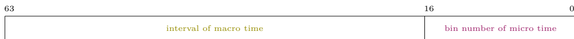
Fig. 3.29: 64 bit data structure of each event processed in LabVIEW, which is saved into a HDF5-file.
