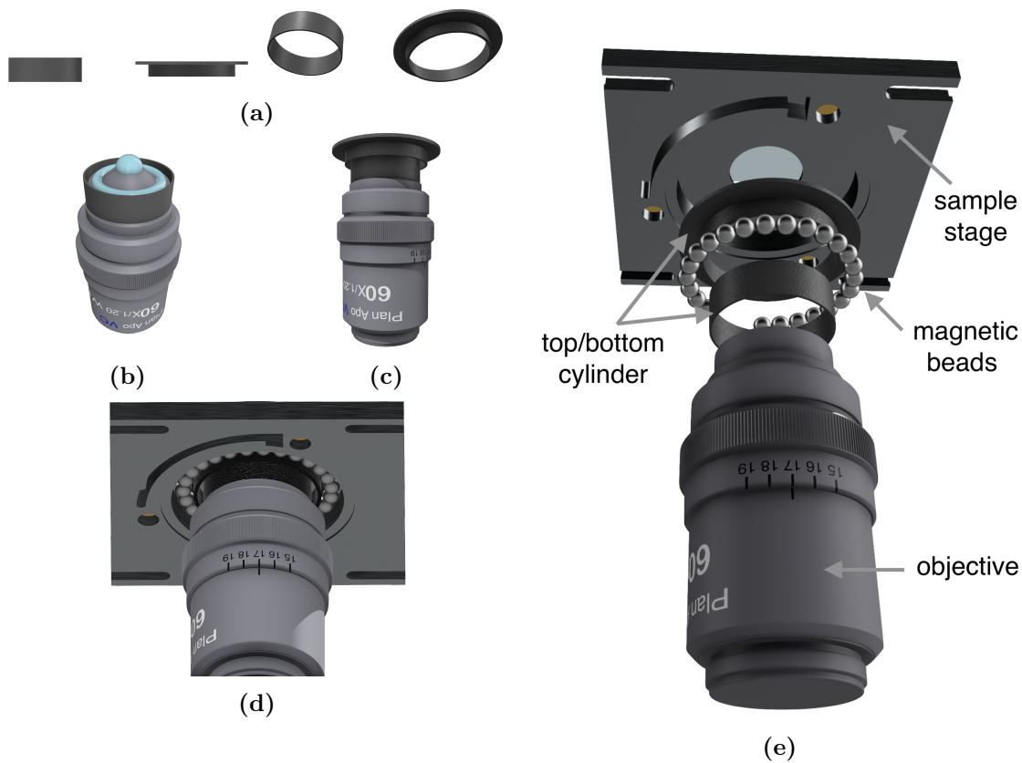
Fig. 4.12: 3D drawing of the immersion water protection device. (a) Two overlaying cylinders prevent an air flow, which would accelerate the evaporation of the immersion water. (b) The bottom cylinder is placed onto the objective. In addition to the immersion water, a little groove of the objective is filled with water to serve as a water reservoir. (c) To create a little chamber, the upper ring is positioned above and (d) is attached to the optical table by magnetic beads. (e) shows all components at once.
