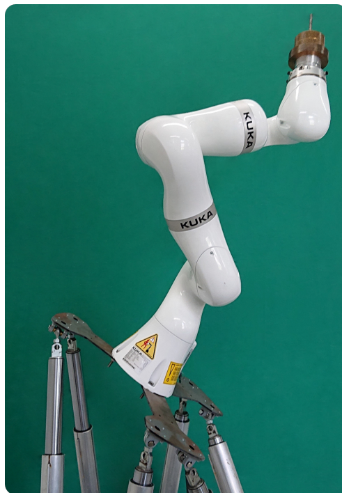
Figure 6.4: The LBR iiwa 7 was mounted on a hexapod to acquire the test data ( dataset_{gen,dir} ), to evaluate the intra-directional generalization performance.
