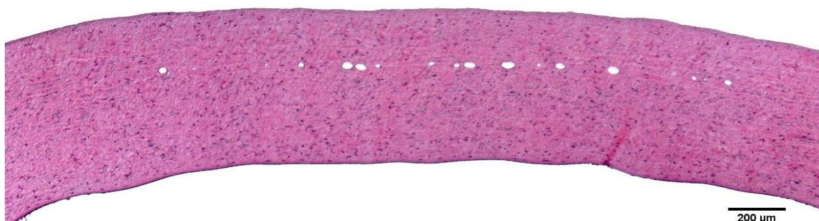
Fig. 3.12. Overview of an intrastromal dissection in 200 \mu\text{m} depth using laser pulses with 355 nm wavelength, 560 ps pulse duration, and 0.69 \mu\text{J} pulse energy focused at NA 0.38 into porcine cornea. Spot separation 4 x 4 \mu\text{m} , Paraffin embedding, H&E staining. Residual bubble are formed within the dissection plane.
