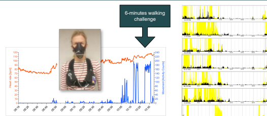
Fig. 2. Energy expenditure assessment during walking by mobile indirect calorimetry
