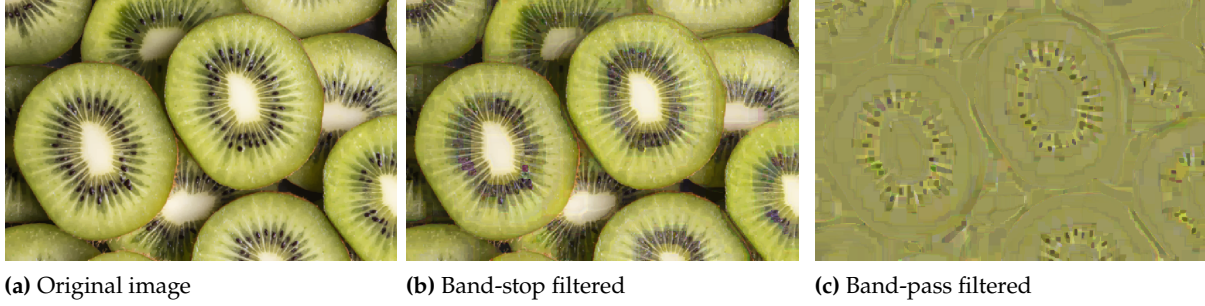
Figure 1.5: Nonlinear Spectral Decompositions. With the help of the inverse scale space flow a nonlinear spectral decomposition (1.27) is defined for images which then allows to define filters (1.28). The filters manipulate the nonlinear eigenfunctions of the regularizer which are contained in the input image according to their eigenvalue (scale). We here show the result of a total variation based band-stop (b) and band-pass (c) filter applied to the input image (a). As indicator functions of certain convex sets are eigenfunctions of the 2D total variation regularizer [BCN02, Thm. 4] edges are well preserved by the filter.
