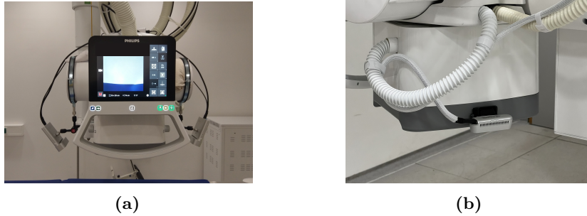
Figure 5.1: In panels (a) and (b) the X-ray source is located in the horizontal tube, while the collimator is contained in the cube below the tube. The experimental setup used to acquire the Clinical Setting Depth Dataset , including the mounted Azure Kinect ToF cameras for acquisition, is shown in panel (a). One camera was mounted at each end of the X-ray tube so that the center of the collimation area is always in the field of view. In panel (b) the setup used to acquire the Clinical Practice Depth Radiograph Dataset , including the Intel DS435i mounted to the back of the collimator, is shown.
