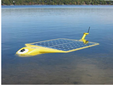
Figure 2.15 The Solar Powered AUV (SAUV) [32]
