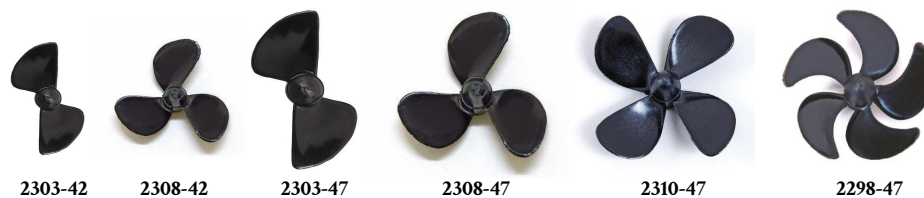
Figure 4.5 The tested propellers with different sizes and blades
