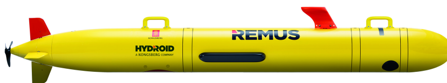
Figure 2.4 REMUS-100 is a 100 meter rated AUV, used with permission from Kongsberg Maritime [117]
