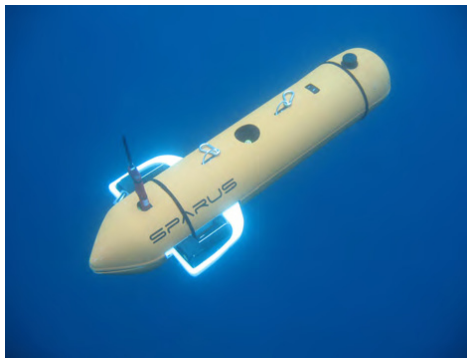
Figure 2.9 Sparus AUV, created in the underwater robotics laboratory at the University of Girona [133]
