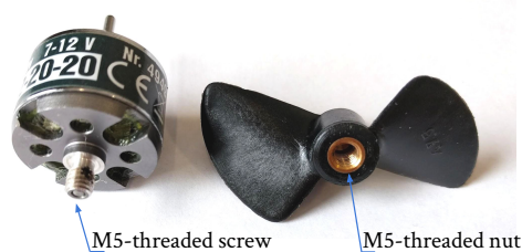
Figure 4.7 The connection between the DC motor and the propeller
