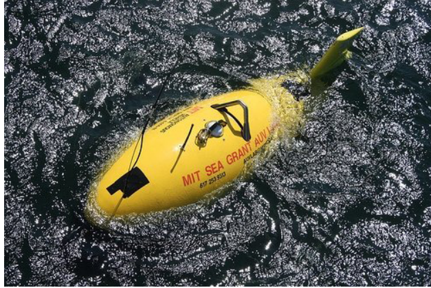
Figure 2.3 Odyssey II class AUV developed at MIT Sea Grant's AUV Lab [143]
