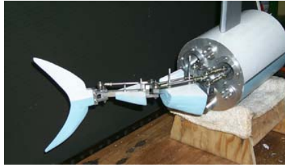
Figure 4.2 A prototype fish robot PF-600 developed to facilitate the investigation of propulsion performance [146]
