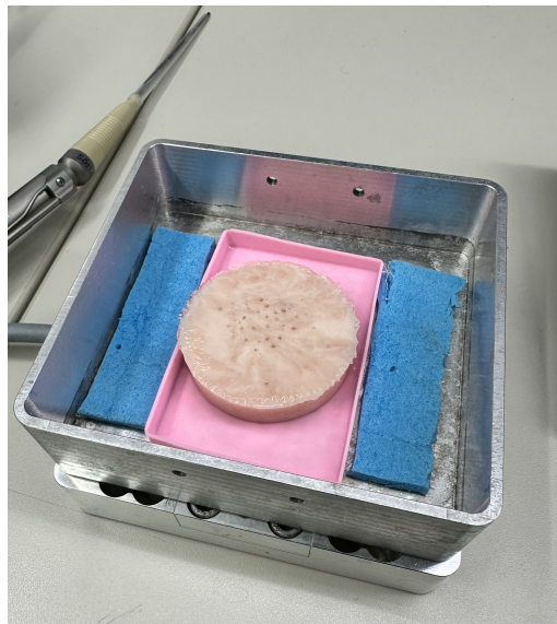
Figure 4.6: Force sensor setup for data acquisition process. Tissue model placed in silicone mold on top of the force sensor located inside a metallic housing. Blue sponges are used for synchronization between electrical and force data.
