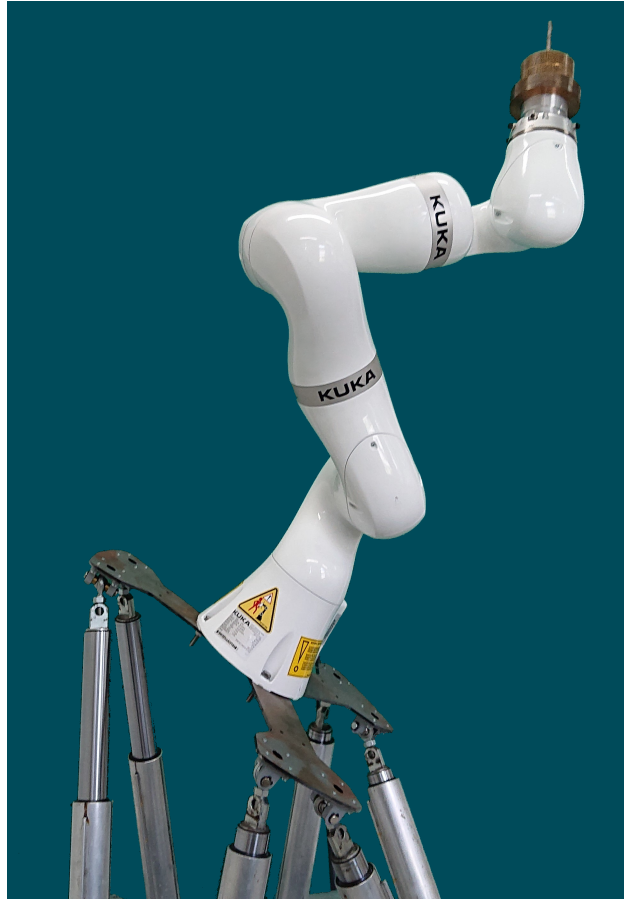
Figure 5.8: The LBR iiwa was mounted on a hexapod to acquire additional test datasets, to evaluate the intra-directional generalization performance.
