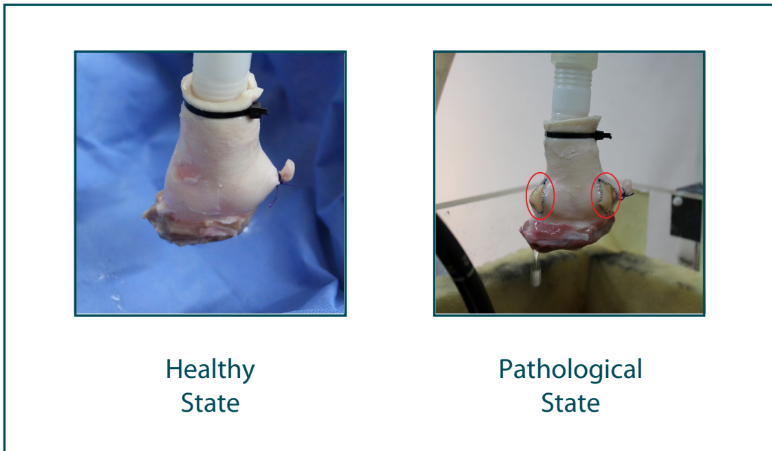
Figure 4.5: Aortic root in the native, healthy state (left) and after manual dilation to simulate a morphological pathology (right). The diamond-shaped patches are encircled in red. Adapted from [62] ©2016 IEEE.
