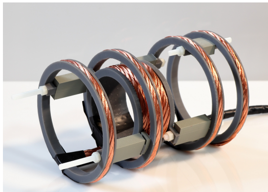
(b) Prototype of the hyperthermia insert. The the coil support parts are printed using Form 2 ( Formlabs, USA) and Ultimaker3 (Ultimaker B.V., Netherlands) 3D printers. The printed parts are assembled together using screws and thread rods.
