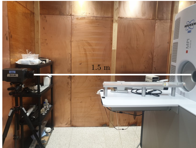
(a) Temperature measurement of the phantom test. A thermal camera is placed 1.5 m away from the opening of the scanner bore.
