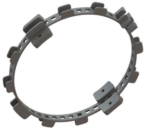
(a) CAD model of the coil support part of one compensation turn.
