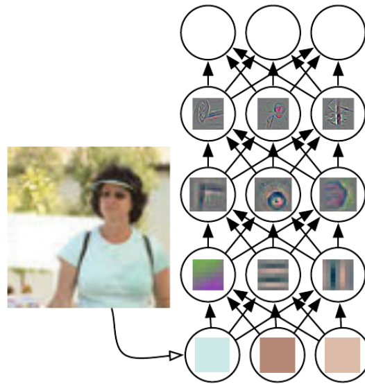
Figure 1.4: Feature hierarchy illustration: a CNN classifies an input image (left) by processing it sequentially with several convolution layers. The bottom circles on the right represent the input pixels of an image, i.e., the visible layer. Each circle above the visible layer symbolizes an artificial neuron of the so-called hidden layers. The small image patches within these circles visualize the features extracted by the neuron (patches based on Zeiler and Fergus [ZF14]). Hence, the neurons of the first hidden layer (right above the visible layer) process the input pixels, extracting features such as lines, edges, and color blobs. Subsequent layers extract increasingly complex features – from corners and edges to object parts. Finally, the output neurons (uppermost circles on the right) can recognize the objects important for the image’s classification. Here, for example, a CNN may classify the input image as ‘person’, distinguishing it from other images showing cars, dogs, or cats. Figure adapted from Goodfellow, Bengio, and Courville [GBC16].
