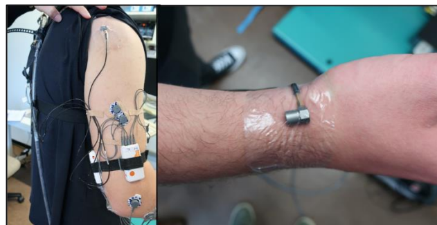
Figure 2.4.3 Unidirectional accelerometer placement. (A) Sensors placed on the lateral humeral condyle (elbow) and acromion (shoulder). (B) Sensor placed on the distal radius (wrist).
