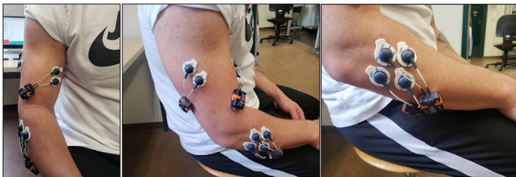
Figure 2.8.2 EMG electrode placement on the exposed arm. (A) Biceps brachii. (B) Triceps brachii. (C) Extensor digitorum (top) and flexor carpi ulnaris (bottom).
