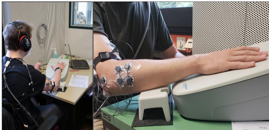
Figure 2.5.1 Finger sensitivity measurement with the VibroSense Meter II. The subject is positioned with their arm loosely extended, elbow slightly flexed, and fingertip placed on the 4 mm thick metal probe.
