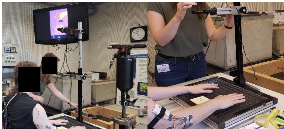
Figure 2.6.2 Infrared thermography (IRT) setup for measuring temperature reaction. The target area is displayed on the monitor for visual confirmation.
