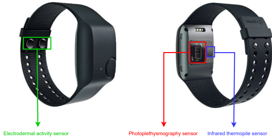
Figure 2.2: Overview of the Empatica E4 wristband (Empatica Inc., Cambridge MA, USA) [84] for the collection of various physiological signals, including highlighting different functional areas related to distinct sensor modalities. It is worth noting that this wearable also holds an accelerometer sensor, but its signals were not utilized due to their irrelevance to this study.
