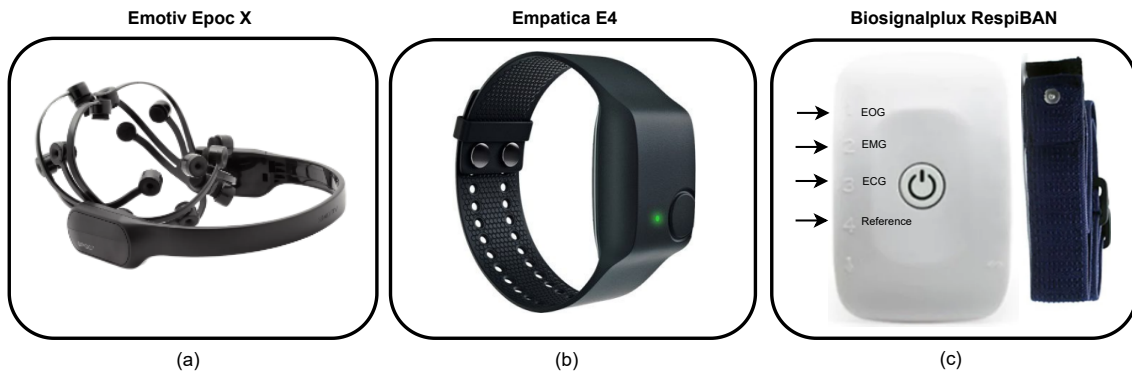
Figure 3.1: List of wearable devices utilized to acquire the physiological measurement of the participants: (a) - Headband style Emotiv Epoc X with 14 electrodes on flexible plastic armbands, (b) - Empatica E4 wristband, and (c) - Biosignalplux RespiBAN wearable device.
