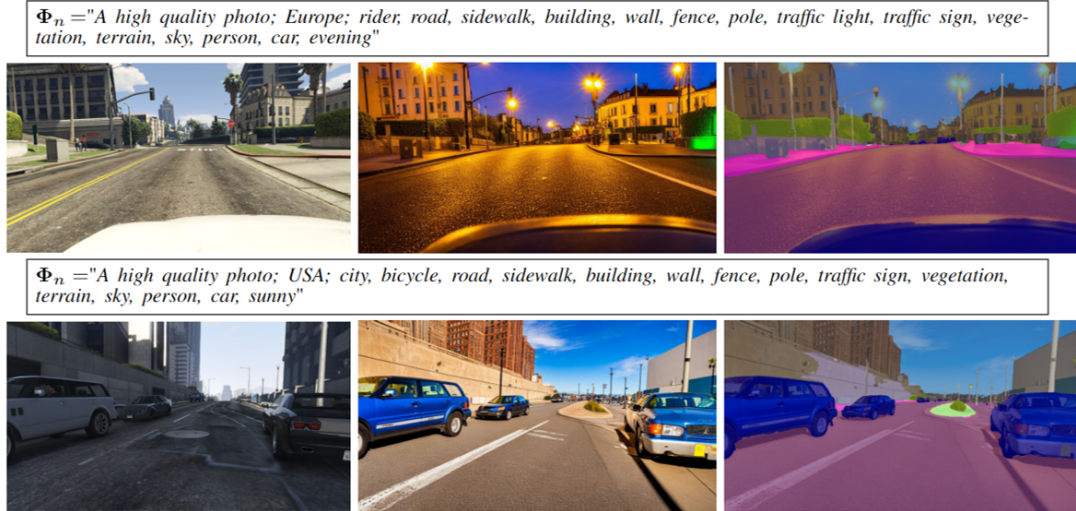
Figure 4.6: Example of utilizing diffusion models to improve realism and quality of a synthetic image. \Phi_n denotes the prompt that, together with the GTA-5 image, serves as input for the diffusion model. A big problem are the semantic inconsistencies created by the generative models (in this case, ControlNet [287]).
